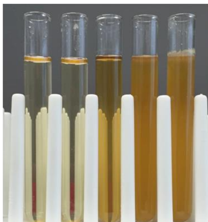
Figure 53. Solvent visual appearance during 500 hour testing (A) Full 500 h timecourse (B) from left: Start of run rich; Start of run lean; End of run lean after being filtered off-line at lab scale; End of run rich; End of run lean.
