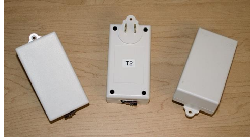
Figure F - 6 – Picture of ZigBee temperature sensor device
