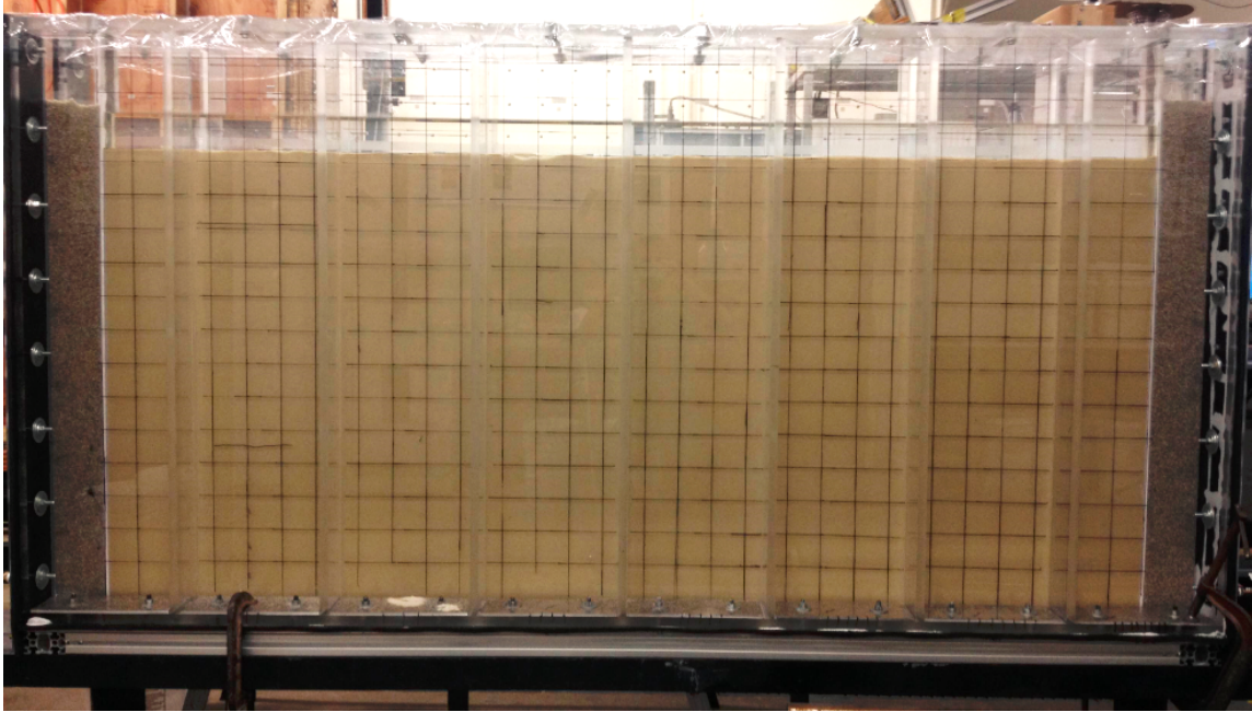
Figure 33 Homogeneous large tank experimental setup showing the sampling grid.
