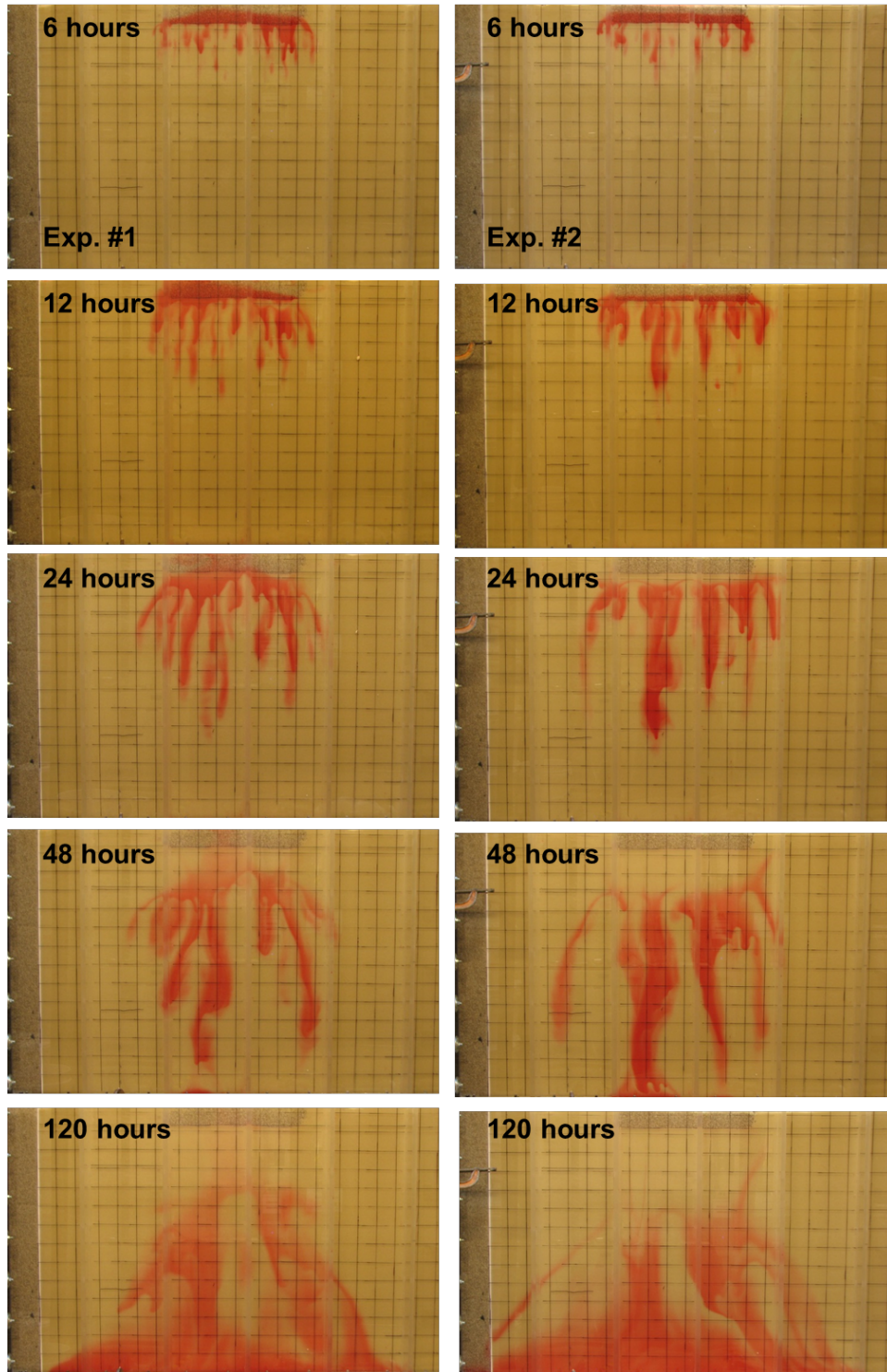
Figure 79 Spreading of density-driven fingers from the front wall for experiment 1 and 2 at (a) 4 hours, (b) 12 hours, (c) 24 hours, (d) 48, and (e) 120 hours after the source release.
