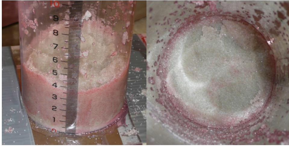
Figure 91 Soltrol penetration along the column wall-sand grain interface at pressures below the entry pressure. No penetration was observed in the bulk of the sand even when Soltrol had penetrated along the interface.
