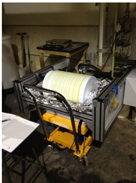
Figure 44. Fiber spools being solvent exchanged with methanol and hexane with a horizontal orientation.
