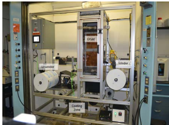
Figure 52. Front view of the continuous hollow fiber coating line.
