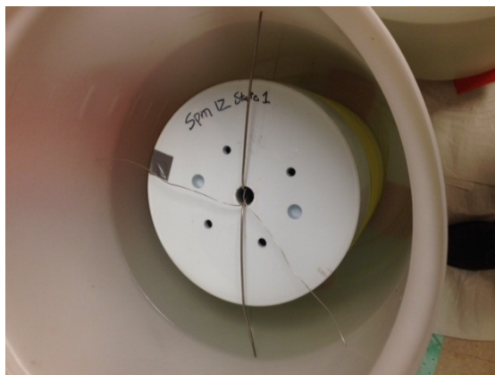
Figure 43. Hollow fiber spool fully submerged in a solvent exchange fluid (water in this case) during the solvent exchange process.
