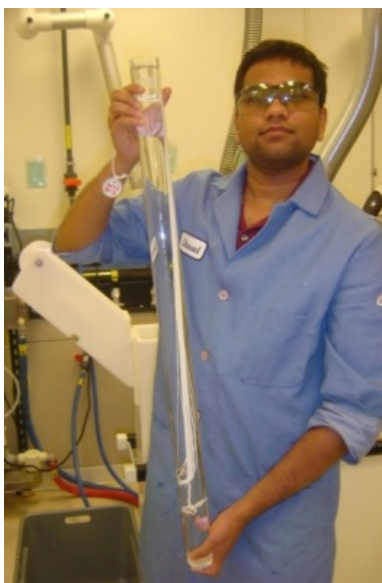
Figure 42. Extruded hollow fiber supports in a solvent exchange tube filled with DI water
