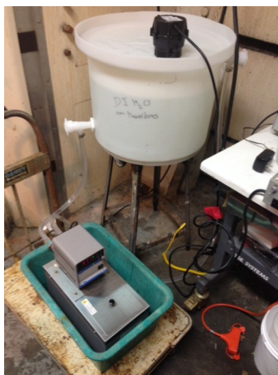
Figure 46. Modified solvent exchange process using fiber lassos with continuous recirculation of warm (40 °C) DI water.
