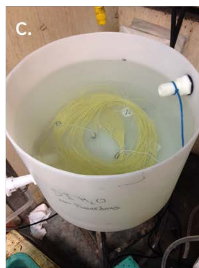
Figure 47. Leaching of possible oligomer and additive (PVP) from the fiber lassos during solvent exchange process. Days 1-2-3 (left to right) are shown for comparison.
