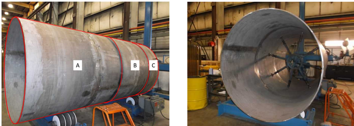
Figure 6: Mock-up container prior to being sectioned. (a) Location of three sections into which the container was cut – one for residual stress analysis (A) and two for specimens (B and C). A temporary spider (b) was placed just below the cut made between sections A and B in order to minimize distortion as the cut was made.
