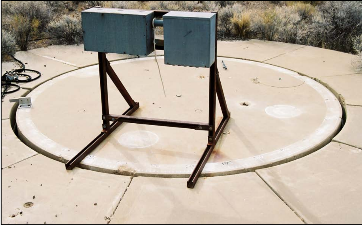
Photo 72. Program 9 equipment and instrumentation were mounted to the turntable stand shown here and rotated into various positions relative to the neutron accelerator mounted on BREN Tower. View to the southeast. Photo taken by DRI on November 1, 2006 (on file at NNSA/NSO Curation Facility).
