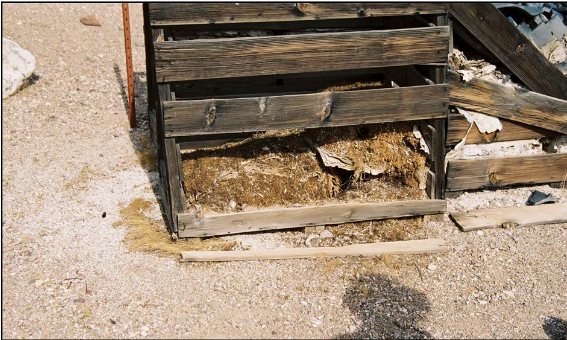
Photo 50. A crate containing seaweed and crushed oyster shell used for the Operation HENRE dosimetry studies conducted on traditional Japanese building materials. Photo taken by DRI on November 1, 2006 (on file at NNSA/NSO Curation Facility).
