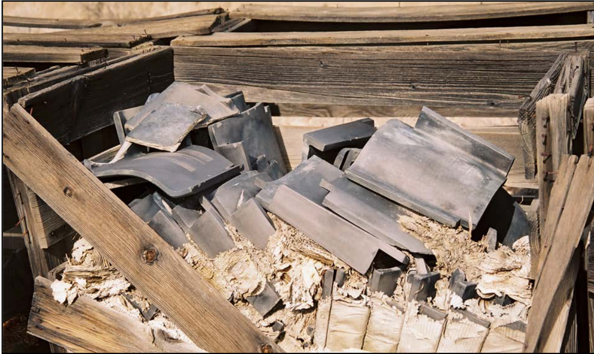
Photo 49. Detail of crate containing ceramic roof tiles used in traditional Japanese construction. The tiles were used for the Operation HENRE dosimetry studies conducted on authentic Japanese building materials. The crate is one of several located near the analog Japanese House. Photo taken by DRI on November 1, 2006 (on file at NNSA/NSO Curation Facility).
