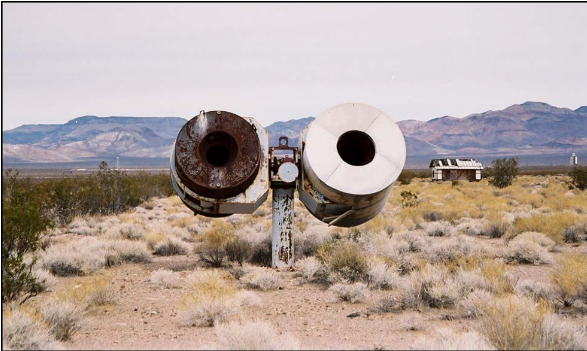
Photo 28. Turreted-mounted collimators located 1,500 ft from BREN Tower. View is to the north. Photo taken by DRI on November 1, 2006 (on file at NNSA/NSO Curation Facility).
