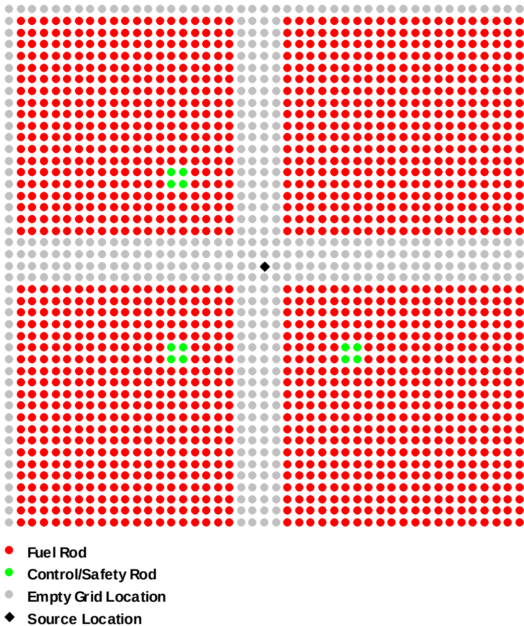
Figure 33. Fuel Rod Layout of the Array Measured for Case 19.
