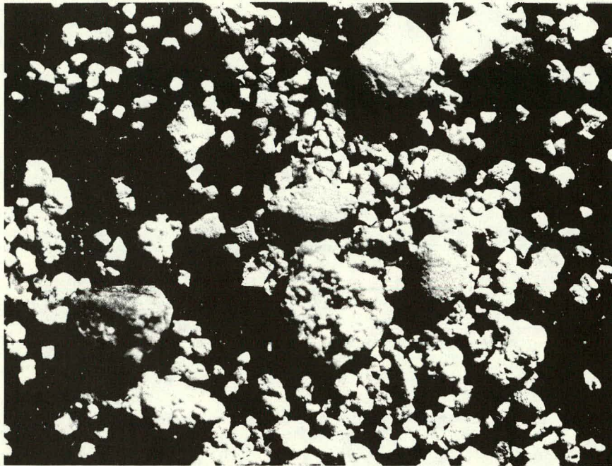
FIGURE 8. +60 MESH FRACTION OF SN502 \text{Si}_3\text{N}_4 POWDER CONTAINING LARGE AGGLOMERATES AND INCLUSIONS
