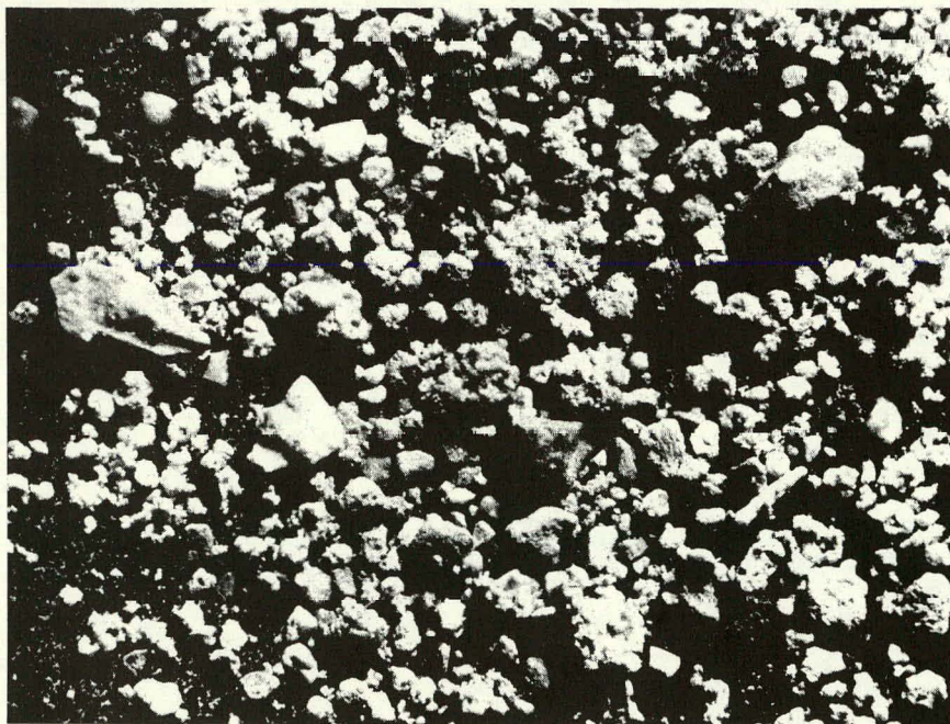
FIGURE 9. +100 MESH FRACTION OF SN502 \text{Si}_3\text{N}_4 POWDER CONTAINING LARGE AGGLOMERATES AND INCLUSIONS
