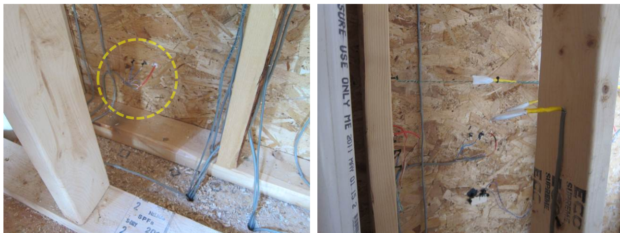
Figure 48. (L) Temperature and MC sensor at sheathing; (R) sensors at mid-height of stud bay
