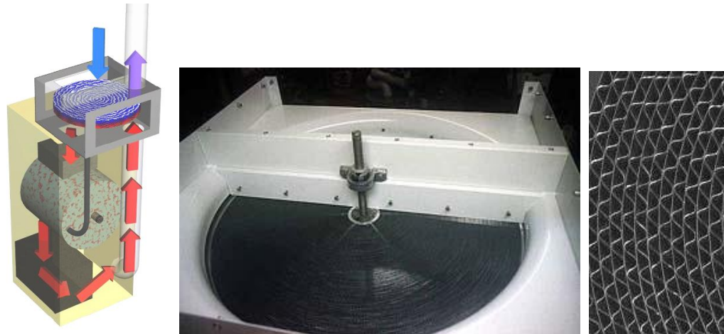
Figure 8-29: Dryer Heat Recovery Wheel Concept
