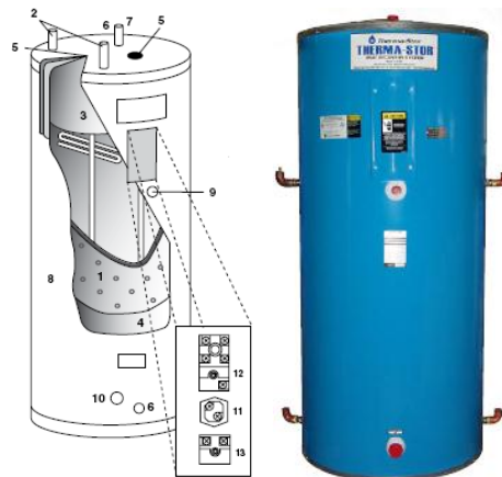
Figure 6-22: Desuperheater Design That Surrounds a Storage Tank Heater, Transferring Heat from the Refrigerant to the Water in the Storage Tank
