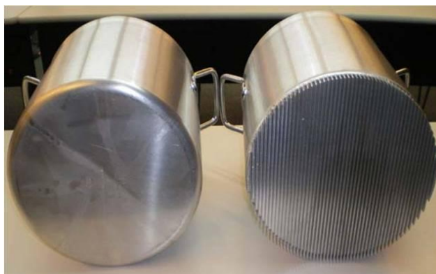
Left: Standard Pot. Right: Pot with Heat Fins Source: Eneron 2009a
