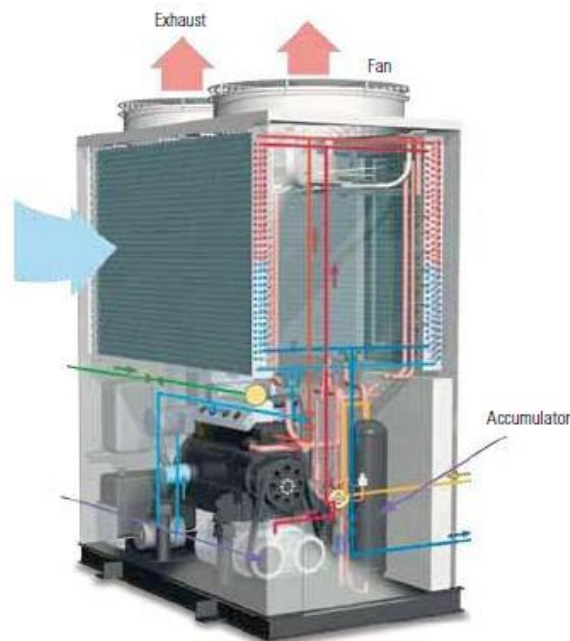
Figure-G.11-1. Typical Outdoor Unit of a Split-System GEHP (10-15 Tons)
