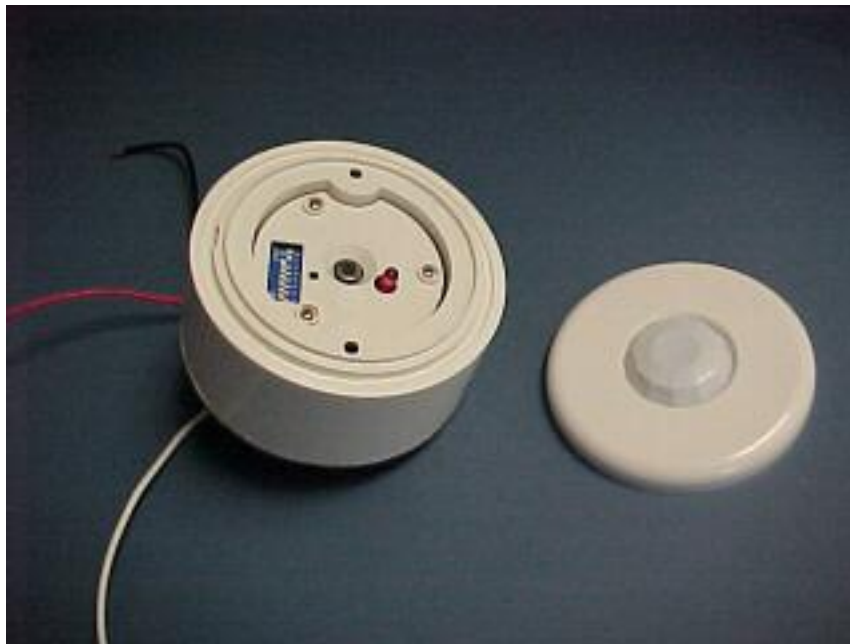
Figure G.24-1. Occupancy Sensor for Smart Ceiling Fan with Fresnel Lens
