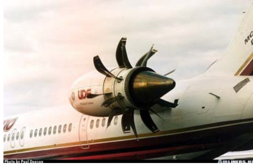
Figure 3.2. Open rotor propulsion
