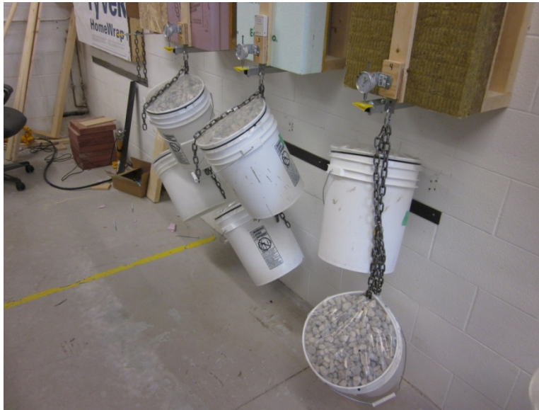
Figure 7. Dead weights attached to bottom edge of furring strips
