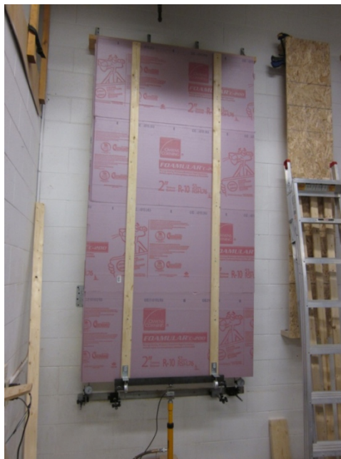
Figure 4. Short-term deflection test panel
