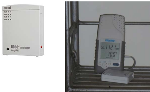
Figure 8. Left: Loggers used for temporary indoor measurements. Right: The loggers have external channels for additional sensors; e.g., for \text{CO}_2 concentration.
