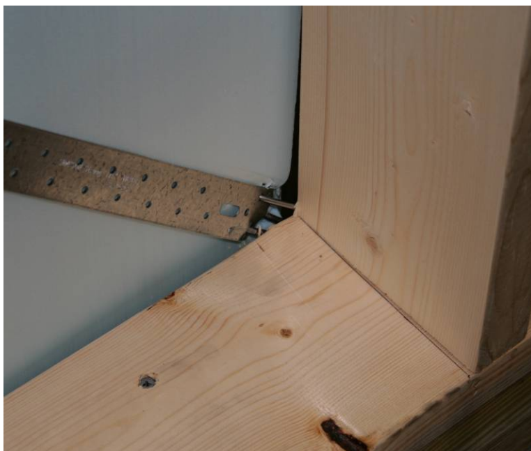
Figure 22. Metal strap nail pullout
