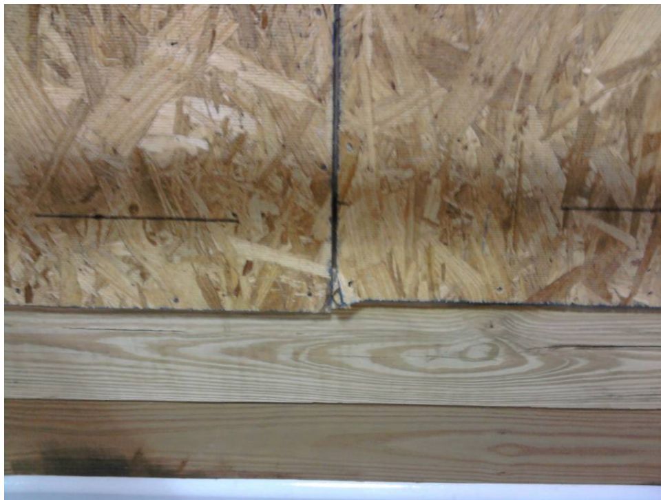
Figure 19. OSB failure at fastener
