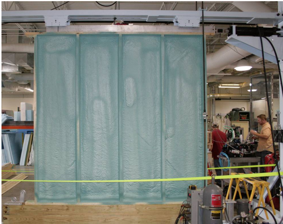
Figure 25. Structural testing wall 2 installed in apparatus
