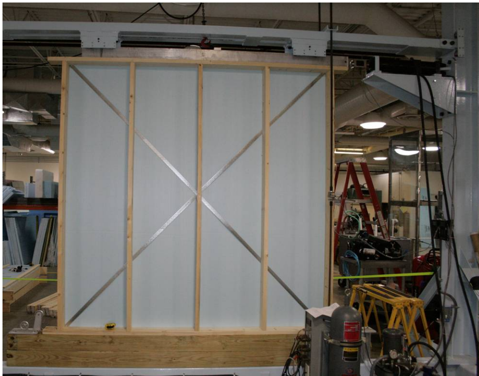
Figure 20. Structural test wall 1 installed in apparatus
