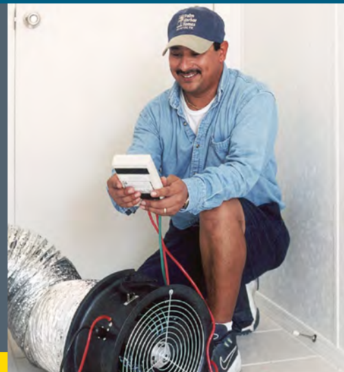
Duct blaster testing confirms that ducts are well sealed ( Photo source: NREL ).
