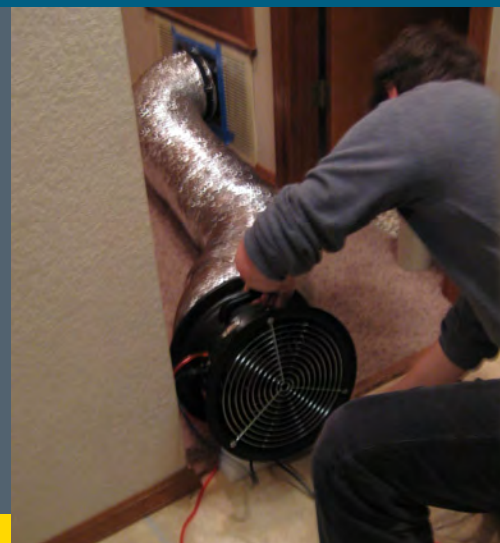
Duct blaster testing confirms that ducts are well sealed ( Photo source: PNNL ).
