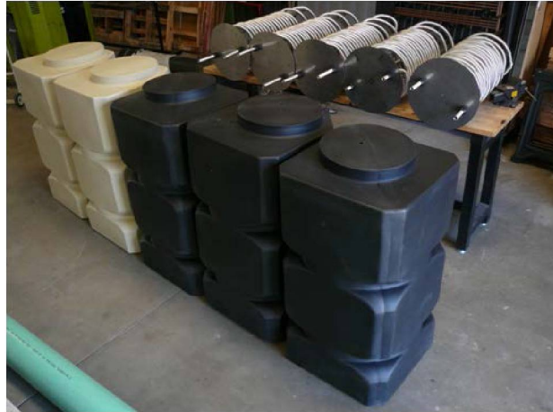
Figure 51. Unpressurized rotomolded tanks with immersed stainless steel HXs
