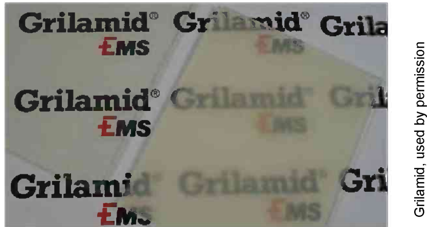
Figure 46. Thermotropic polyamide in clear and scattering states
