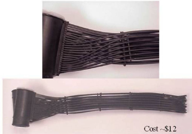
Figure 44. Prototype low-cost polymer HX. Tubes are \frac{1}{8} in. (3 mm) diameter. Tube production, tube weaving, and tube-to-header welding are automated processes, contributing to a low-cost projection.
