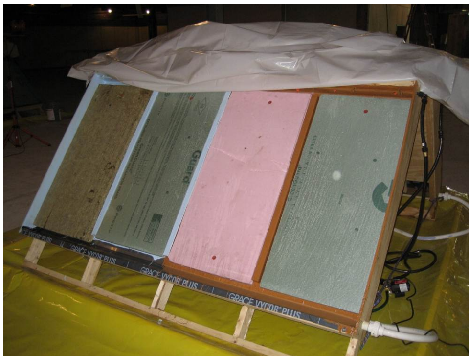
Figure 18. Drainage testing durability spray rack
