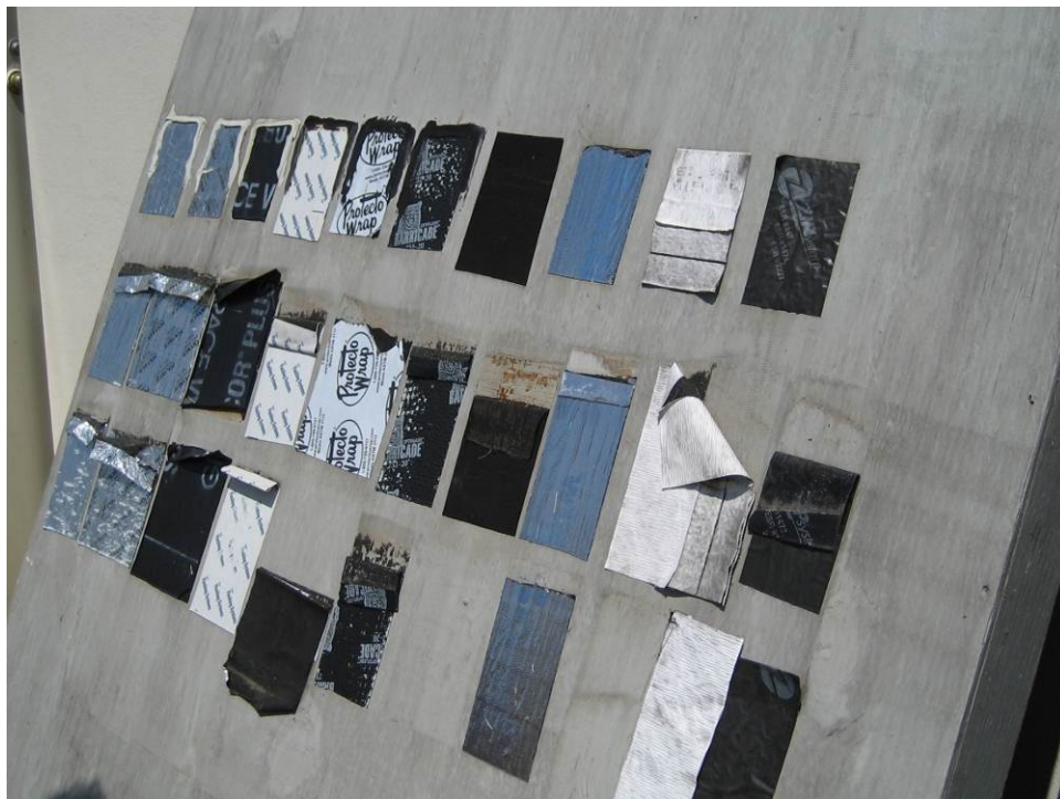
Figure 21. Exposure testing of peel and stick membranes
