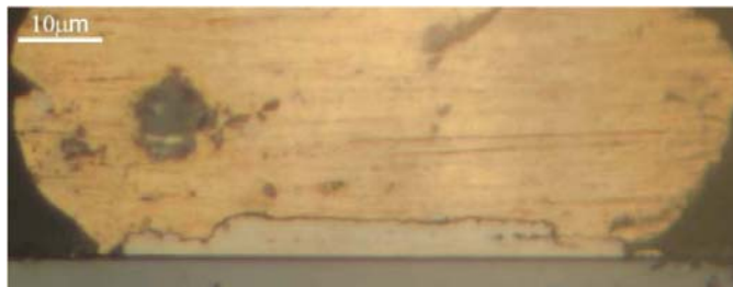
Figure 6. Intermetallic formation between Au wire and Al bond pad
