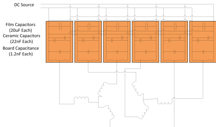
Fig. 8. Controller architecture for demonstrator 10 kW IMMD drive.
