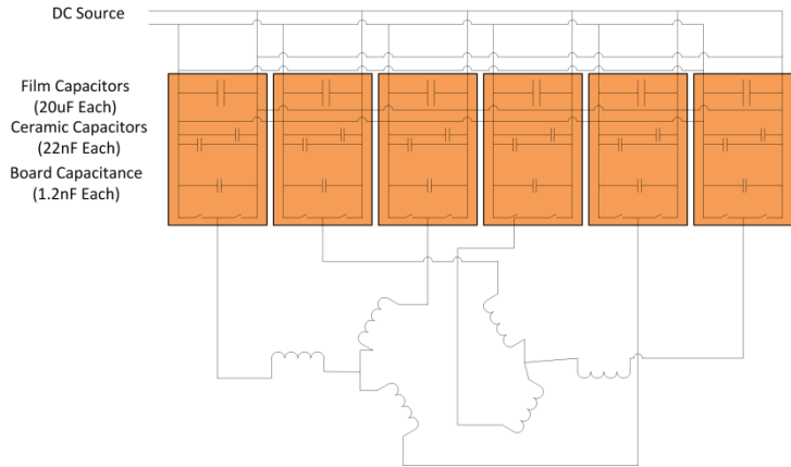
Fig. 7. Power circuit schematic for demonstrator 10 kW IMMD drive.
