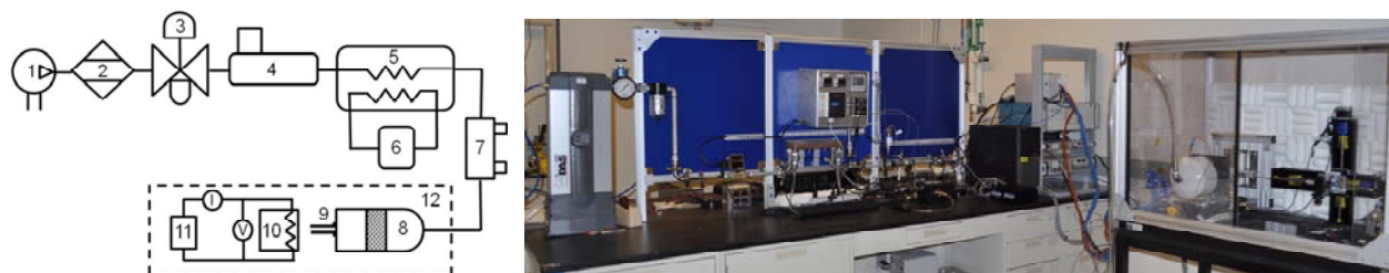
Figure 8. Schematic and photograph of the steady jet experimental setup: (1) compressed air, (2) desiccant dryer, (3) filter/regulator, (4) mass flow controller, (5) plate heat exchanger, (6) recirculating bath, (7) laminar flow element, (8) settling chamber, (9) nozzle, (10) heater target, (11) heater power supply, (12) isolation box
