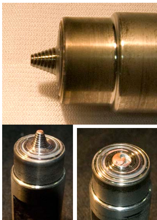
Figure 1. Many process conditions tested led to tool probe failure due to the drop in yield strength of the tool material at high temperatures
