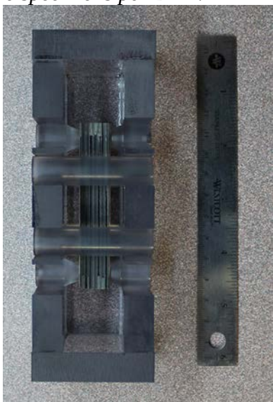
Figure 6. Top view of four-point-bend fixture for testing the sector flexure specimen. A specimen is shown positioned under the top two rollers.
