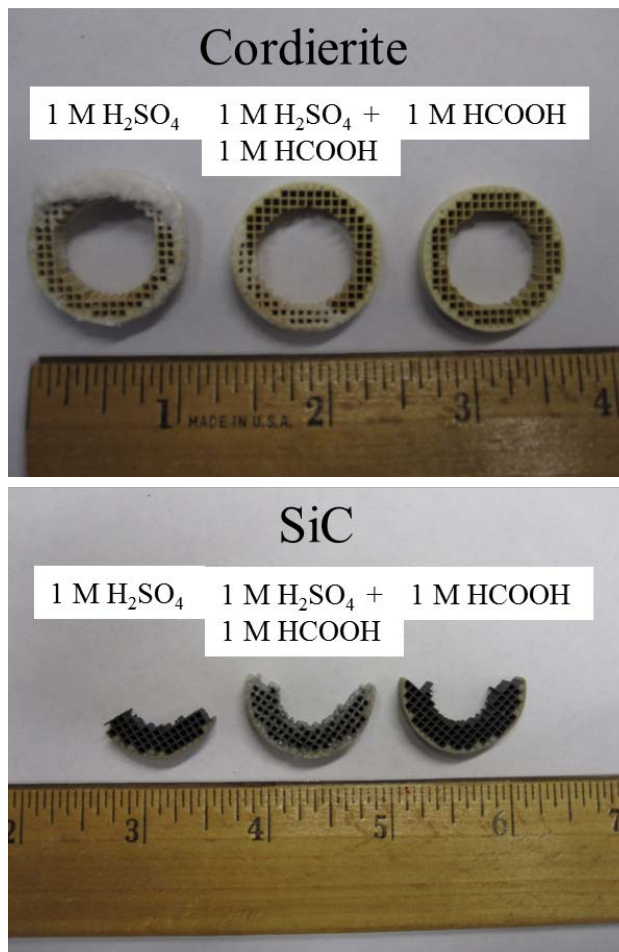
Figure 13. Chemically-attacked DPF samples. The cordierite sample following sulfuric acid attack shows significant amounts of \text{Al}_2(\text{SO}_4)_3 .
