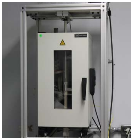
Figure 3. Medium-temperature furnace surrounding bend test set up.
