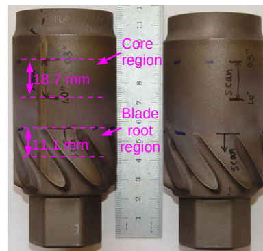
Figure 14. Two machined cylindrical core samples of TiAl turbine wheels.
