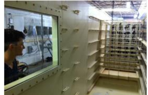
THOR's Open Channel Re-Circulating Ocean Current Flume. Water depth speed profiles can be tailored to simulate various flow conditions.
