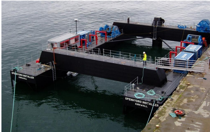
3. Once on the seabed, the lifting lines are released and the Deployment Vehicle is towed back to harbour.
