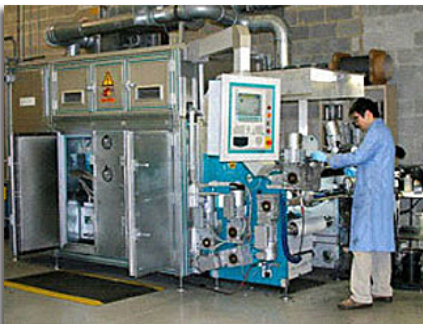
BASF Coating Machine for MEAs
