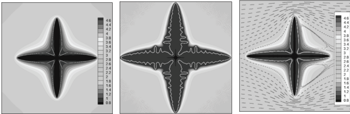
Figure 2. Dendrite morphology and solute map with various boundary conditions: (a) solute diffusion only, (b) constant heat flux at boundaries, (c) constant inflow velocity at left side, and (d) inflow velocity and constant heat flux at boundaries.
