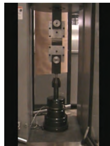
Figure 2. TMAC tension setup for testing the ACC super lap shear weld-bond specimen.
