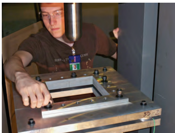
Figure 3. Flat-panel test setup for ballistic toughness testing on TMAC.
