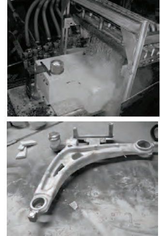
Figure 1. Ablation process: (a) ablation of a mold in progress; (b) ablation of control arm complete.
