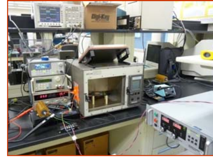
Fig. 1. High temperature gate driver test setup.
