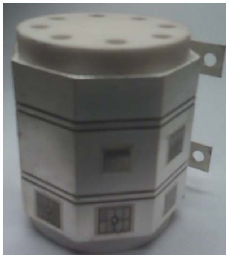
Fig. 12. Nickel-/silver-plated part with IGBTs and diodes sintered into position.
