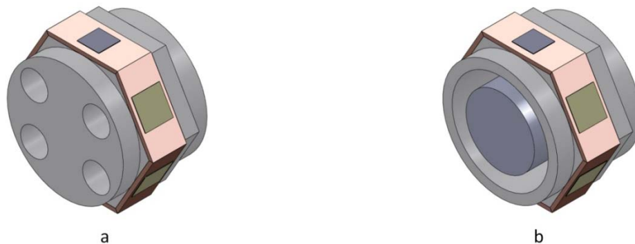
Fig. 33. Isometric view of package configurations with both cooling options: (a) Four-hole cooling design, (b) Annulus cooling design
