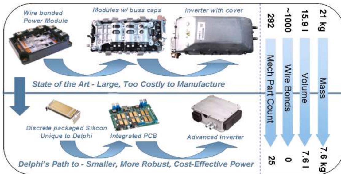
Fig. 6. Delphi's Power Technology Path to Smaller, Lighter, Manufacturable and Lower Cost Power Electronics
