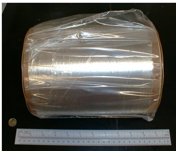
Fig. 2. Spool of the high temperature polymer dielectric produced at ECI
