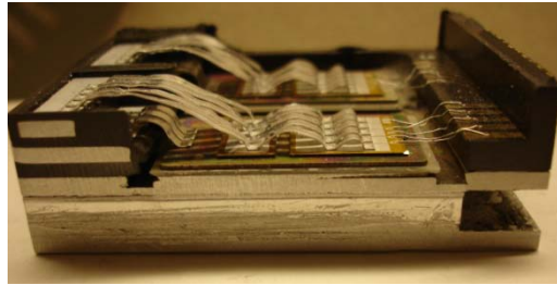
Fig. 5. Cross-section of boost converter modules 2010 Prius.
