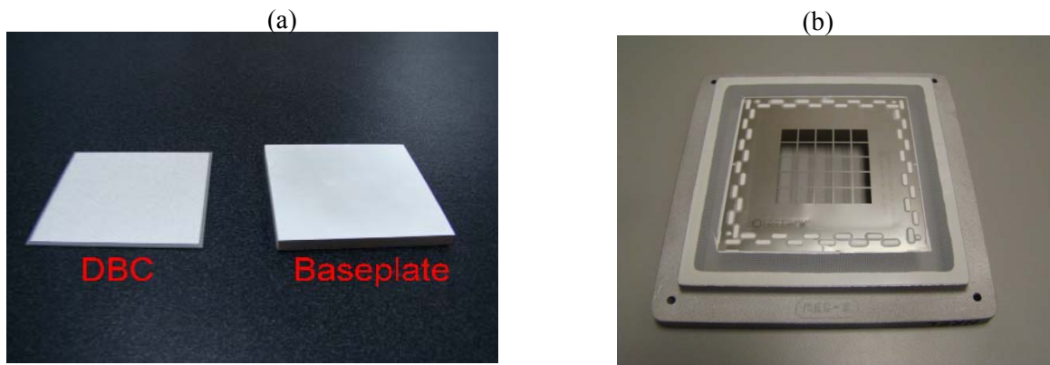
Fig. 53. (a) Sample DBC substrate and base plate, (b) Stencil for printing pastes
