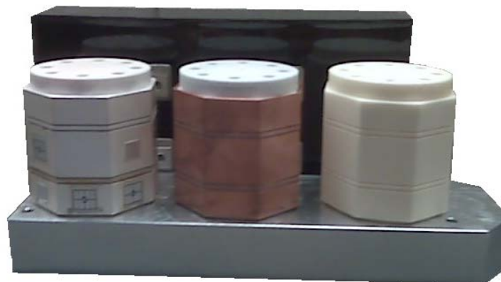
Fig. 15. Inverter assembly buildup as of September 24, 2010 (top flow header removed).
