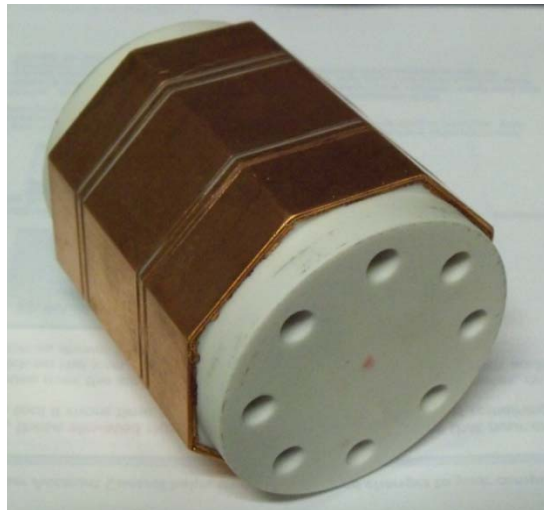
Fig. 10. Final component bonded with copper by Stellar Industries.
