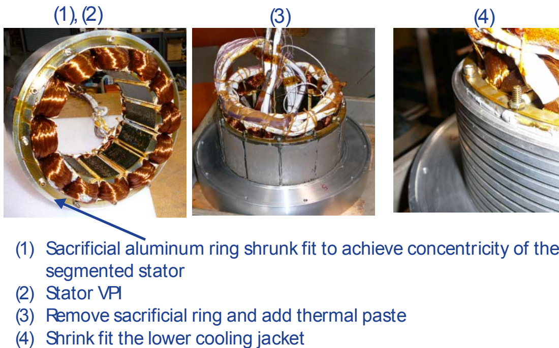
Fig. 9. Assembly steps to improve contact between the cooling jacket and the stator outer diameter
