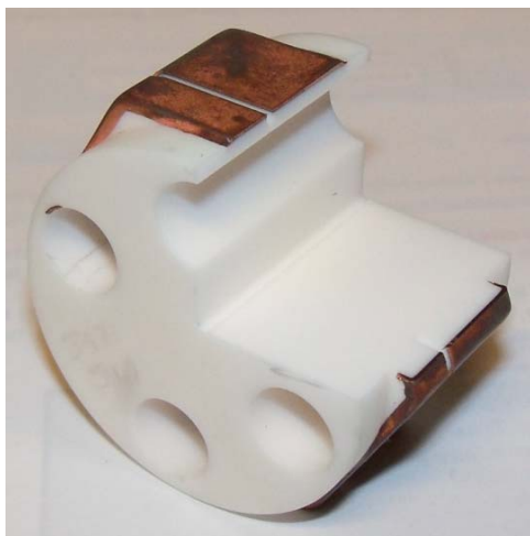
Fig. 7. Sectioned part used for copper bond evaluation.
