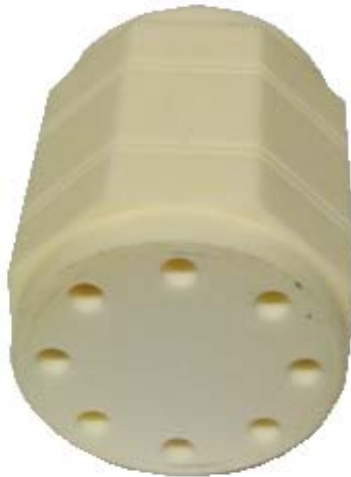
Fig. 9. Finished alumina octagonal substrate fabricated by CoorsTek.
