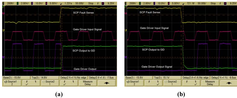
Fig. 9. SCP test results at 175°C of current fault: (a) fault “ON”; (b) fault “OFF.”
