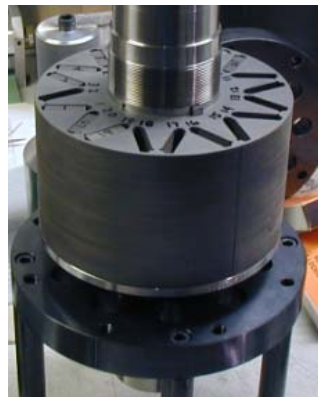
Fig. 10. Rotor of the second proof-of-principle machine
