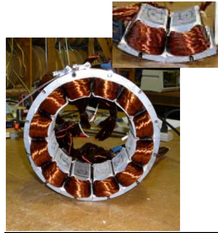
Fig. 2. Stator of the first proof-of-principle machine
