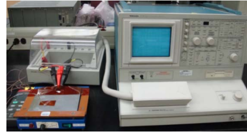
Fig. 10. Static characterization setup with curve tracer.
