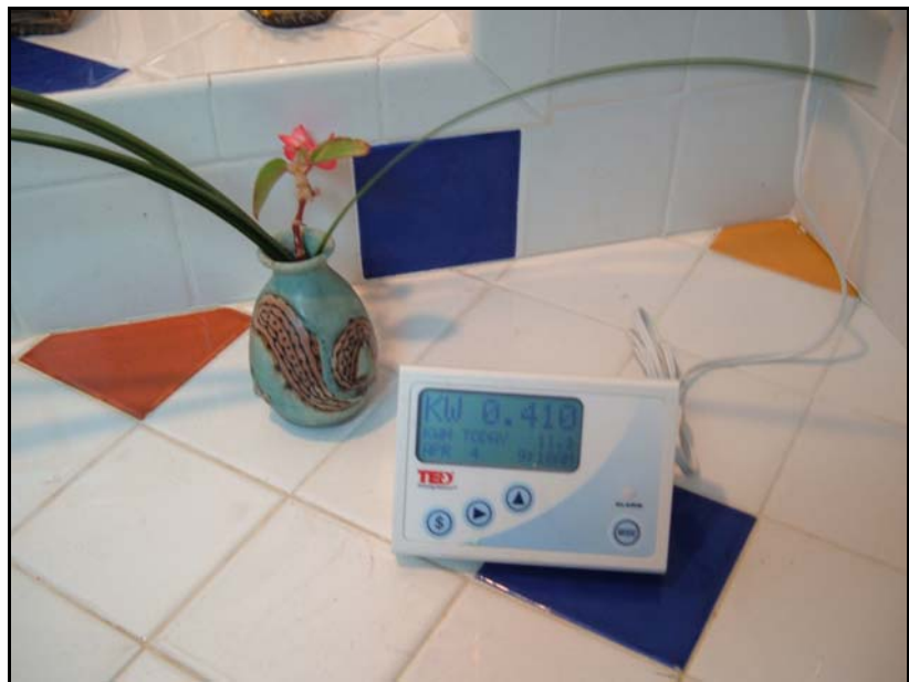
Figure 3. Free standing display of The Energy Detective (TED) feedback device. Display shows house is currently drawing 0.410 kW.
