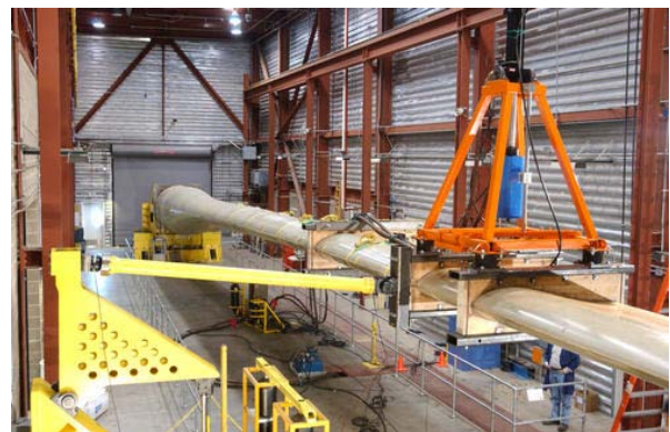
Figure 6. Blade undergoing structural testing
