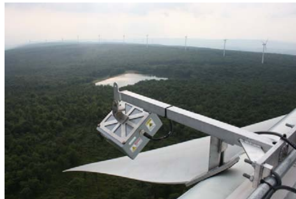
Figure 66. Experimental acoustic bat deterrent device
