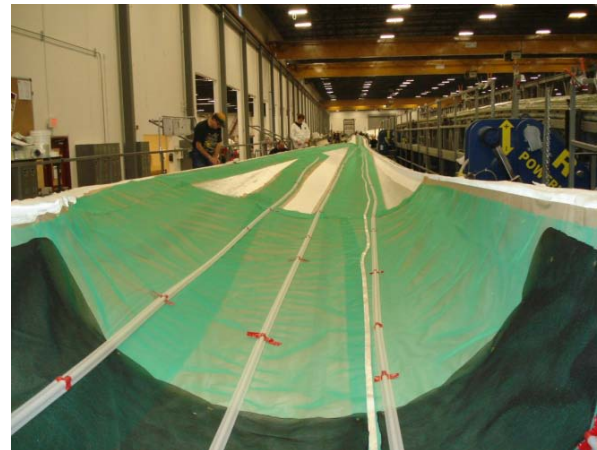
Figure 25. Blade manufacturing lay-up
