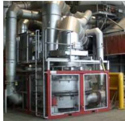
Figure 7 - (a) Rotary Regenerator (Source: PG&E, 1997), (b) Rotary Regenerator on a Melting Furnace (Source: Jasper GmbH, 2007)
