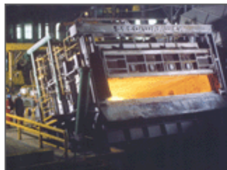
Figure 25 - Gas-Fired Aluminum - Reverberatory Tilting Furnace - (Source: Seco/Warwick Corporation)
