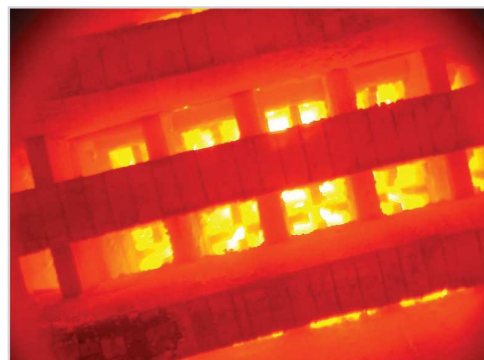
Figure 6 - (a) Regenerative Furnace Diagram, (b) Checkerwork in Glass Regenerative Furnace (Source: GS Energy & Environment, 2007)
