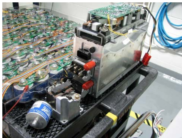
Figure 11. 60-kW (peak) Brusa BDC412 DC/DC Converter.
