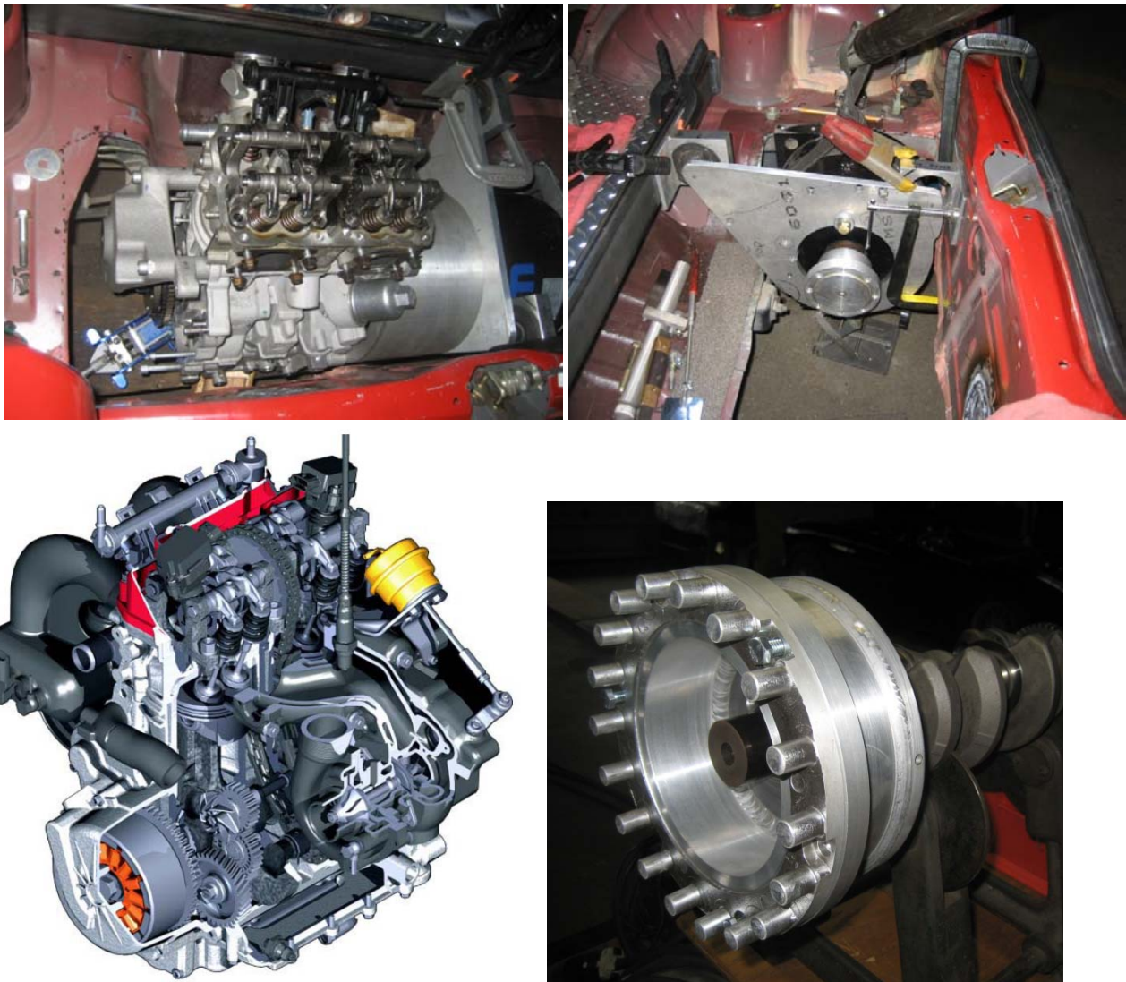
Figure 19. Weber 2-Cylinder 750 cc Displacement Engine
