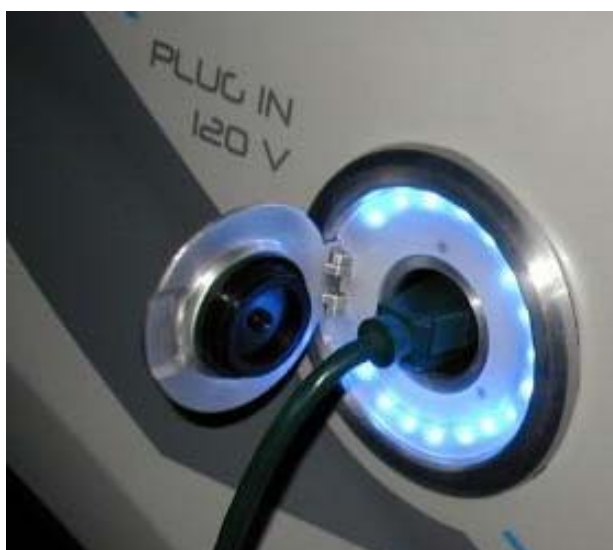
Figure 2. Ford E85 PHEV Escape's unique 120-Volt Charge Port Located in the Front Left Side Fender, in Use
