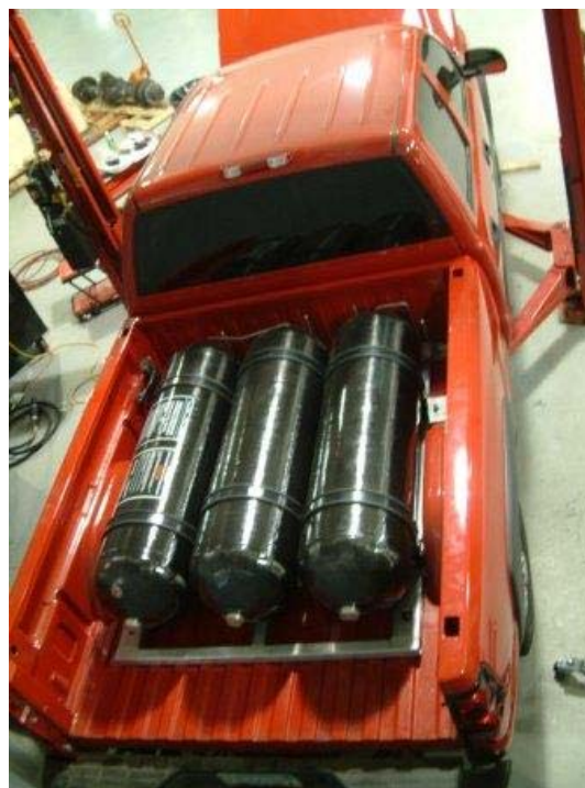
Figure 2. Dynetek Hydrogen Fuel Tanks in the Bed of the Pickup
