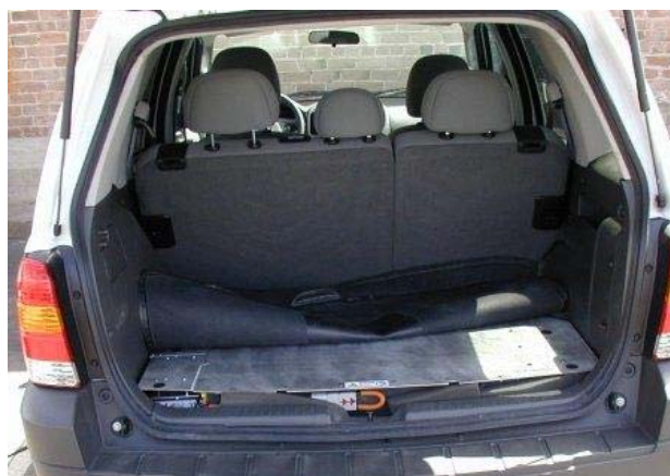
Figure 9. Hybrids Plus PHEV conversion of a Ford Escape: The Hybrids Plus battery pack is under the metal cover, allowing full use of the rear storage area.
