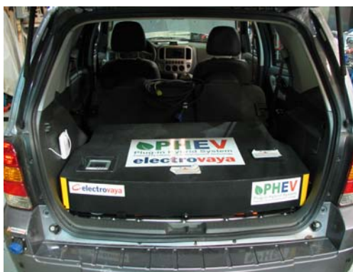
Figure 2. Battery System of the Electrovaya Escape PHEV
