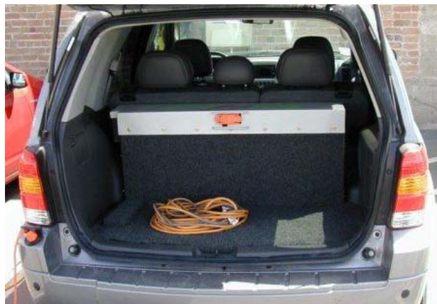
Figure 7. A123 Lithium Ion Battery Pack Placement in the Hymotion conversion of a Ford Escape: The pack sits close the back site of the Escape in the rear storage area. A PHEV suitable charging infrastructure extension cord is in the back storage area. The pack is topped by the silver colored metal
