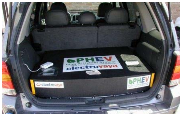
Figure 8. Electroveya Lithium Battery Pack in a Ford Escape converted by Electroveya: The pack takes up the entire rear storage area.
