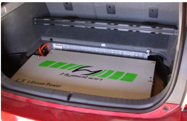
Figure 6. A123 Lithium Ion Battery Pack Placement in the Hymotion conversion of a Toyota Prius: The pack sits between the rear of the vehicle and the original Prius battery, which is retained and used. (The Prius battery is to the right of the bright orange cables and only the upper rear side is visible as bright metal. )
