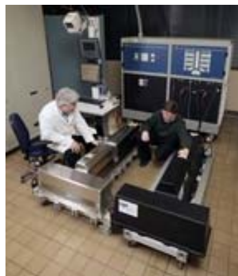
Figure 1. View of Chevy Volt Battery Pack
