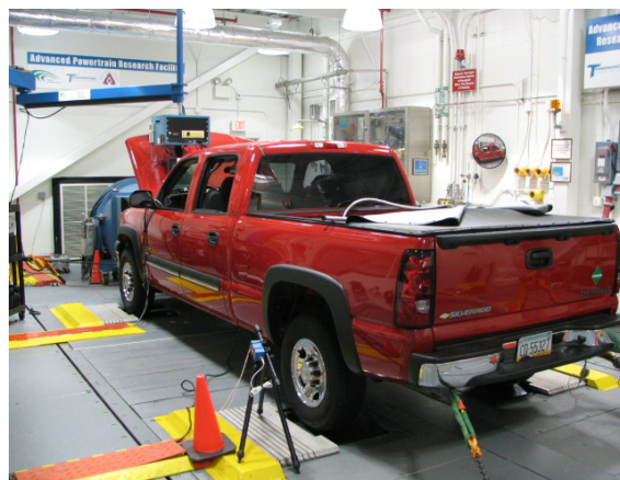
Figure 1. Hydrogen-Converted Truck Undergoing Tests at the APRF
