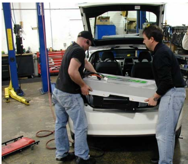
Figure 5. Prius being converted to a PHEV by Hymotion Staff
