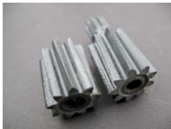
Figure 4. Photograph of the erosion of the polymeric gears after 700 hrs of testing with water containing 2 vol.% SiC nanoparticles
