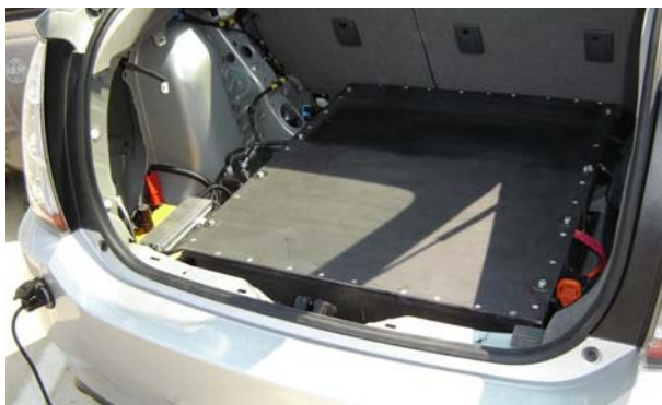
Figure 4. Lithium Ion Battery Pack Placement in the EnergyCS conversion of a Toyota Prius: The pack is in the black box. Note the 110-volt connector cord in the bottom left of the picture.
