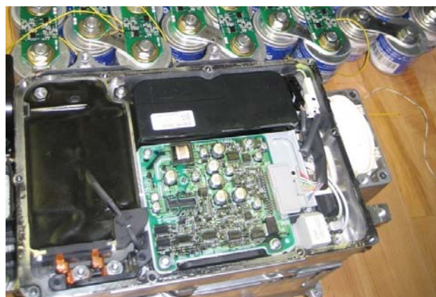
Figure 12. Toyota Camry 35-kW DC/DC Converter
