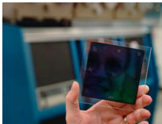
Figure 1. Pictured is NREL#6A solar selective coating deposited by directly and reactively evaporating the layers by elemental co-deposition.
