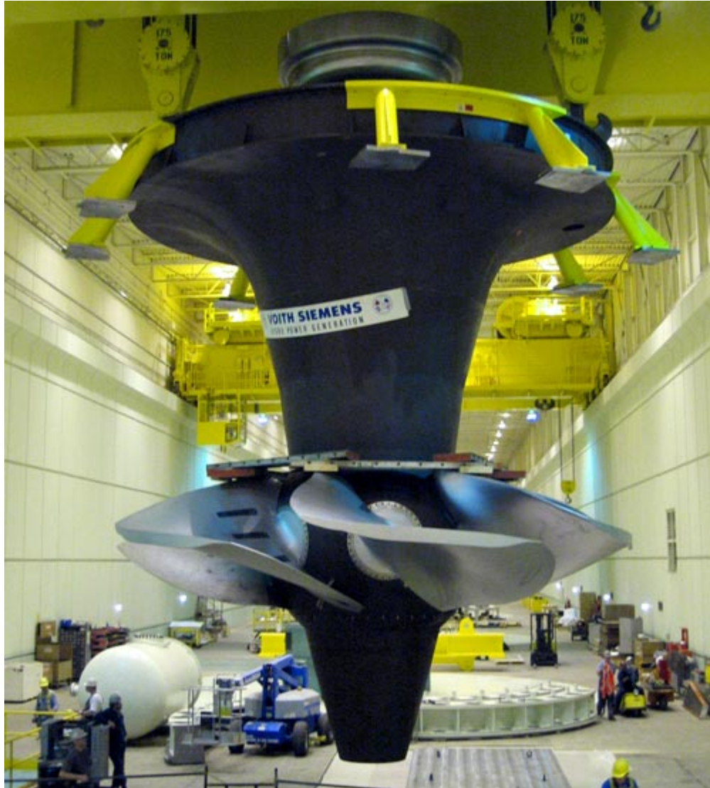
Figure 1.2. Advanced hydroelectric turbine, the Minimum Gap Runner (MGR) that was installed into Unit 8 of Wanapum Dam in 2005.
