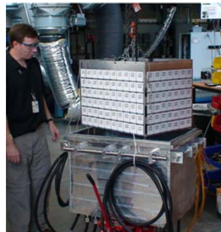
Figure II-5. Internal enclosure of test chamber with heat flux sensors being placed in the external enclosure.
