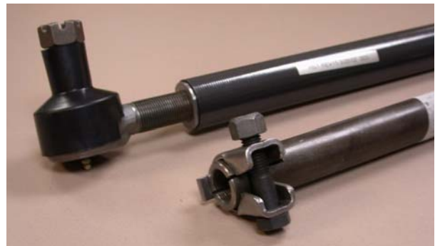
Figure 6. Composite suspension component commercialized for heavy vehicle steer axles.
