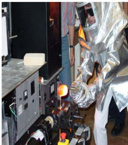
Figure 2. Glass ceramic sheet formation by pouring molten glass on a roller. The sheets made by this process were provided to TRS Technologies for incorporation into a multilayer capacitor.
