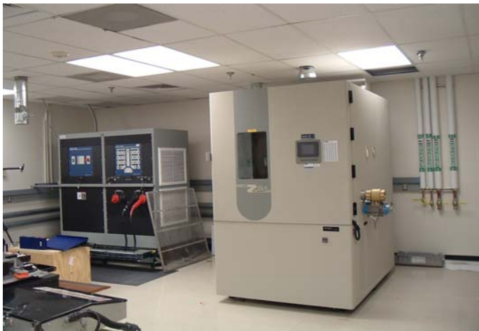
Figure 1. Environmental Chamber and ABC100—125-kW bi-directional power supply
