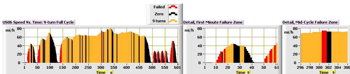
Figure 8(a). US06 cycle failed zones of EV with 9-turn motor.
