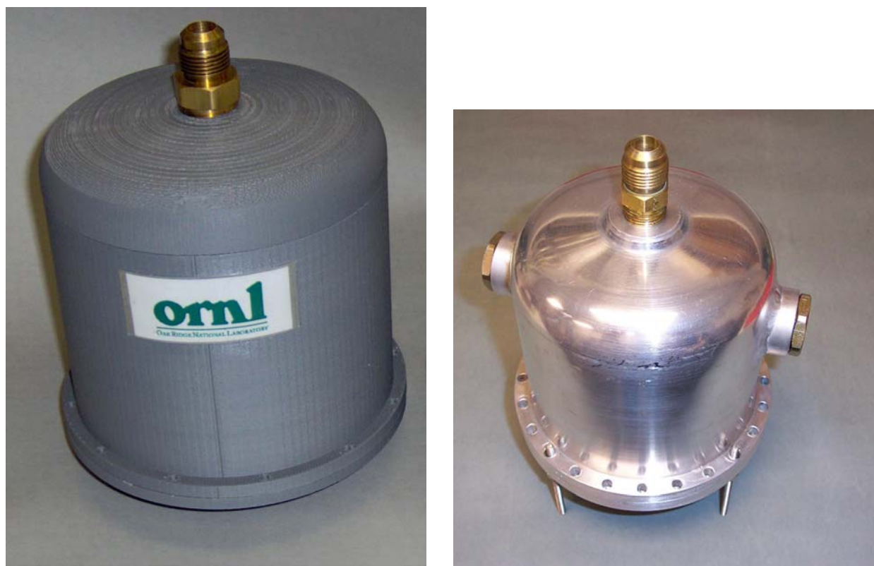
Figure 1. Comparison of FY 2006 inverter model to completed FY 2007 inverter and housing.
