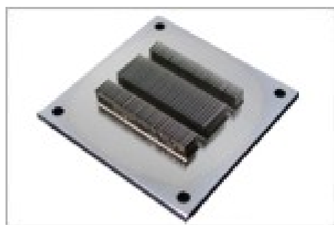
Figure 3. Photographs of micro-channel and micro-jet devices
