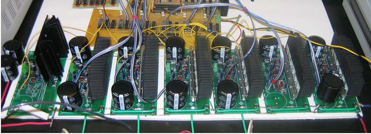
Figure 7. The six-level 5-kW version of the MMCCC with six modules. The sixth module (first one from right) is bypassed for normal operation.
