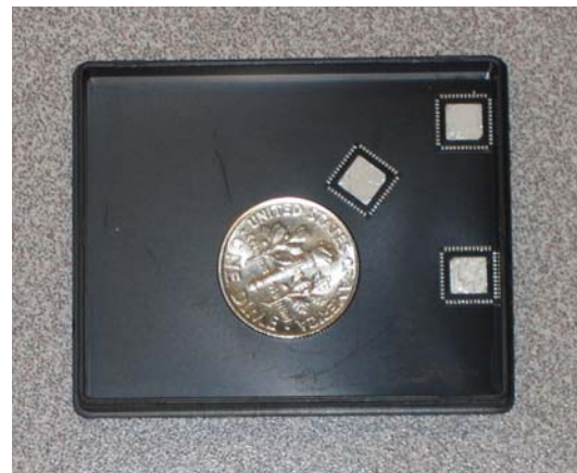
Figure 10. Gate driver IC in CDIL44 package in comparison with a dime.
