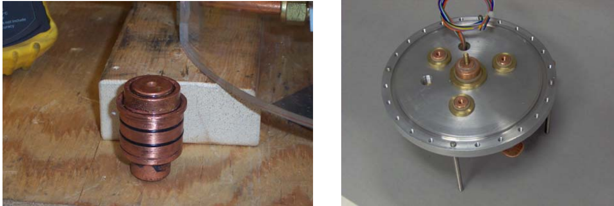
Figure 3. Left shows the two-conductor copper-glass-copper dc link feedthrough. Right shows the bottom flange of the FY 2007 inverter with epoxy-based ac and dc feedthroughs.
