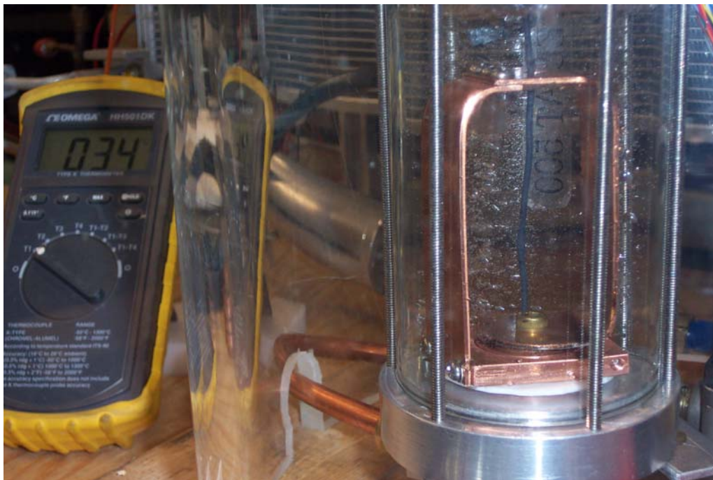
Figure 4. Glass-sealed copper feedthrough testing in R134a at 400 amps.
