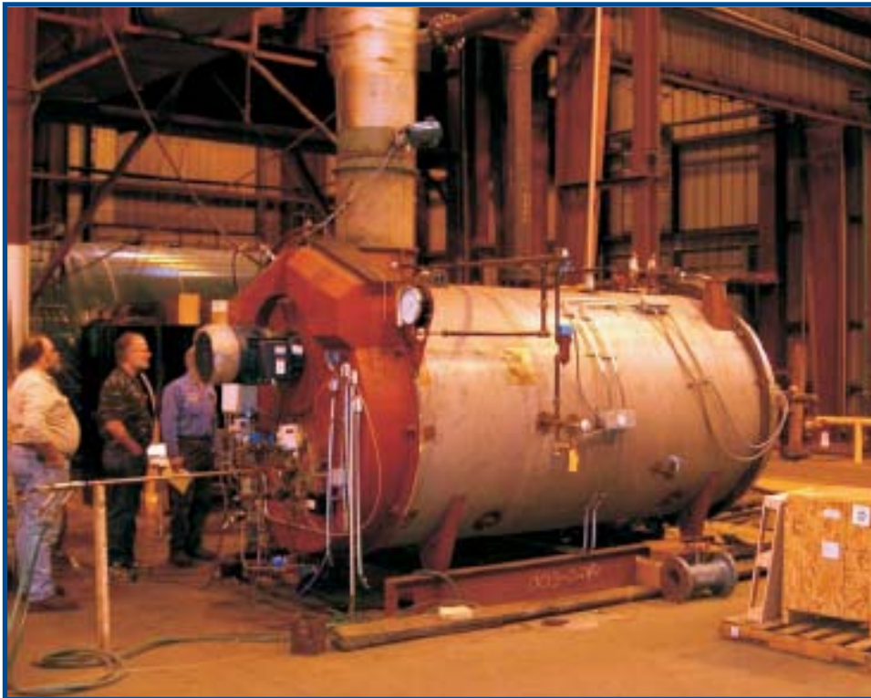
Fig. 1 Two-stage design Super Boiler at Cleaver-Brooks Thomasville Plant.
