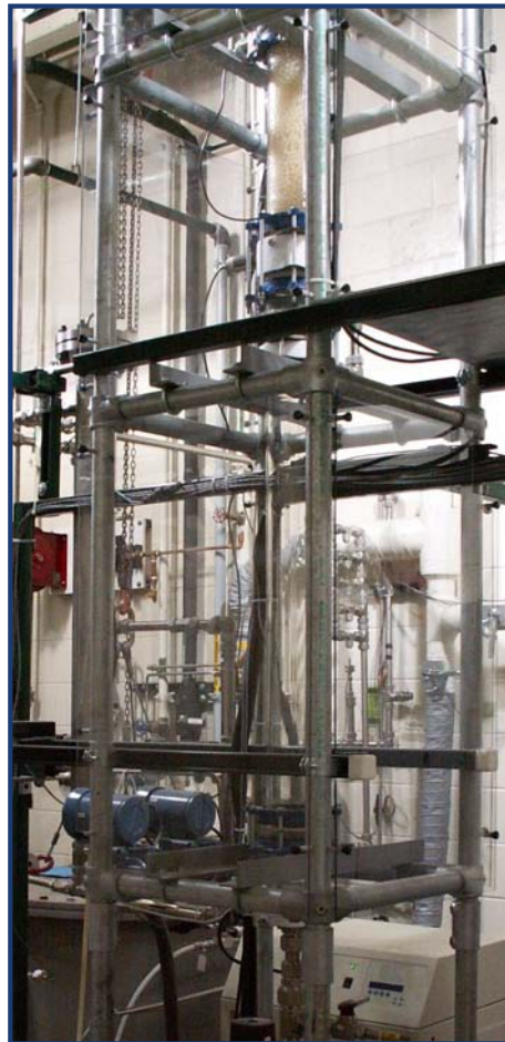
Sandia's Slurry Bubble-Column Reactor (SBCR) testbed. Over the last decade, Sandia's Slurry Bubble-Column Reactor (SBCR) testbed has been successfully used to support indirect liquefaction studies.
