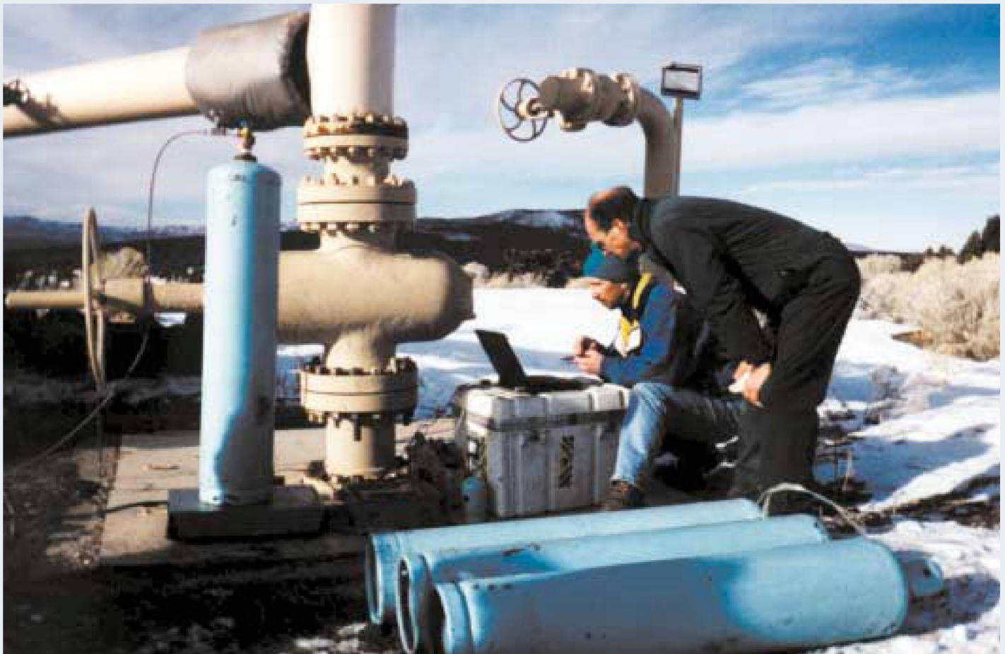
Researchers with the University of Utah's Energy & Geoscience Institute conduct a tracer test at The Geysers.
