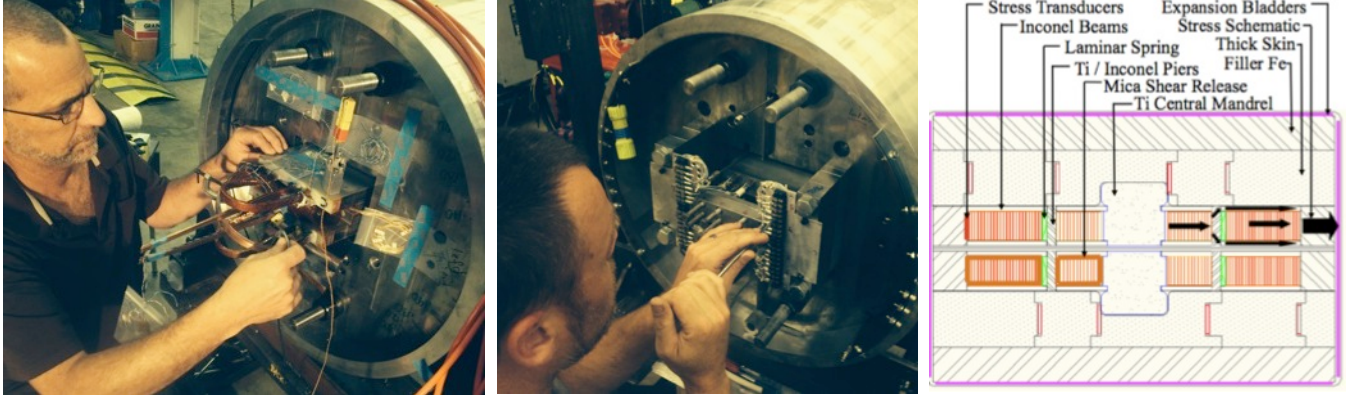
Figure 1. TAMU3 dipole: a) final splices of NbTi leads to interconnect windings; b) installation of H-bridge supporting strain gages monitoring the coil ends; cross-section showing elements of stress management.
