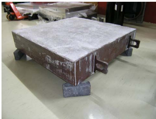
Figure 1. Concrete shield block.
