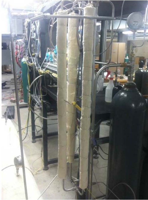
Figure 12. Preheater consisting of three heated and insulated pipes in parallel controlled via PID in Labview.
