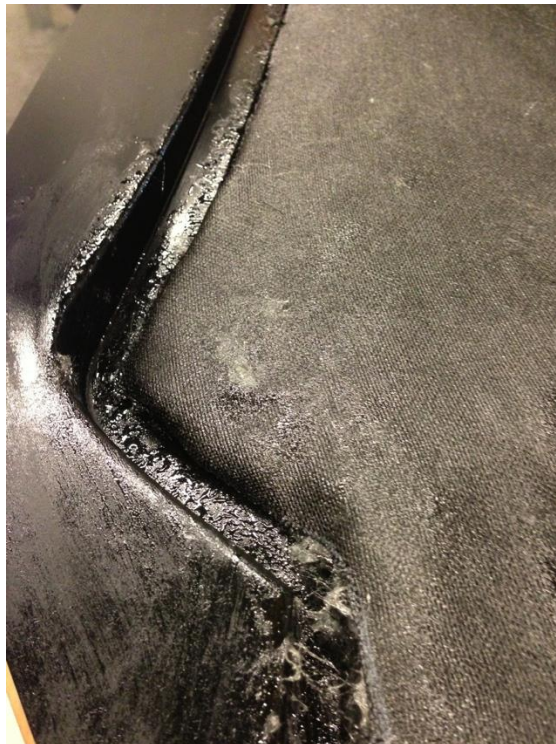
Figure 56 – Leading Edge Prior to Tool Closing
