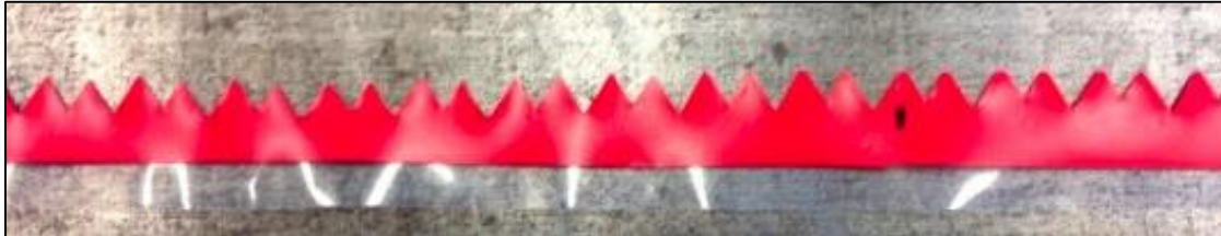
Figure 74 - Boundary Layer Trip
