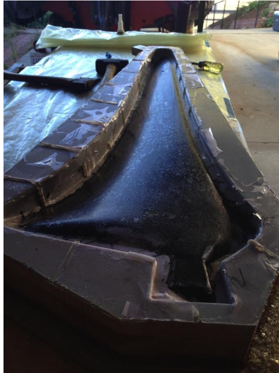
Figure 58 - Blade during De-Molding
