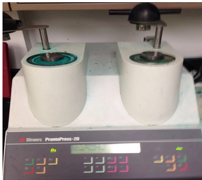
Figure 2.3.1.2. Struers ProntoPress-20 sample mounting machine
