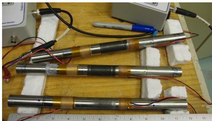
Figure 2.2.2.12. Photographs of experimental setup and specimens (as received, 71% ad 58%).
