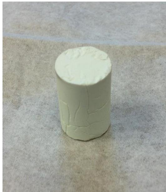
**FIGURE B6** | Sample 2 cm long, sintered under controlled atmosphere.
