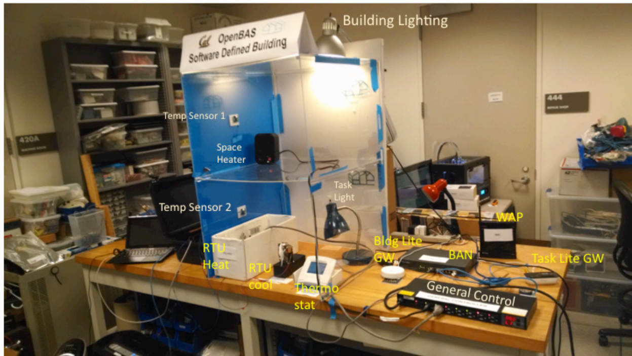
Figure 12: Lab-scale test bed for OpenBAS demonstration of integrated HVAC, lighting, and general control.
