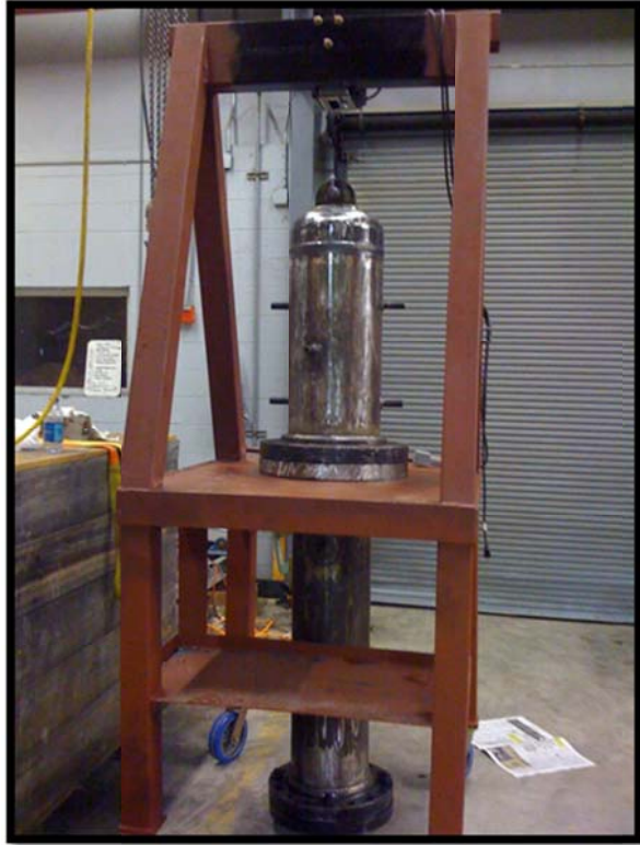
Fig.4.1.2 Thermal cycling test rig under construction (L) and under operation in the lab (R)
