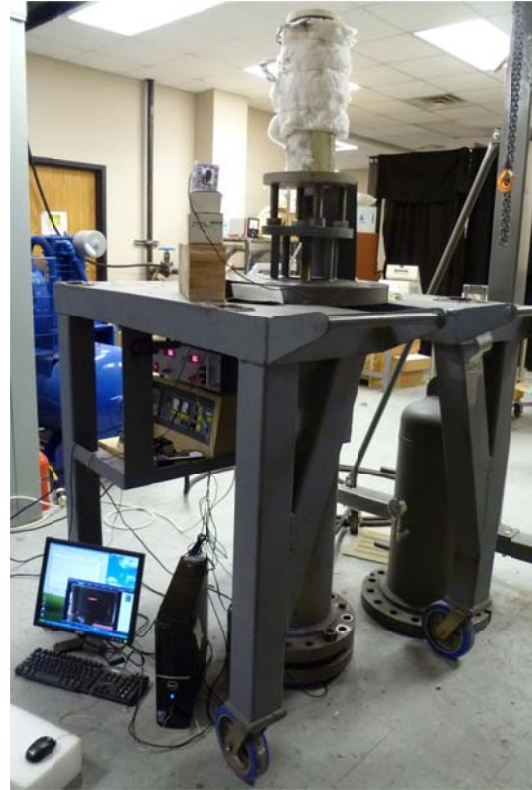
Fig.4.1.2 Thermal cycling test rig under construction (L) and under operation in the lab (R)
