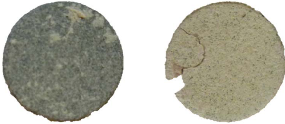
Fig. 4.7.8 Photograph of the failed GZ/GZ50%/YSZ coating after 8 cycles of 10h-thermal-cycling test at 1150 °C.
