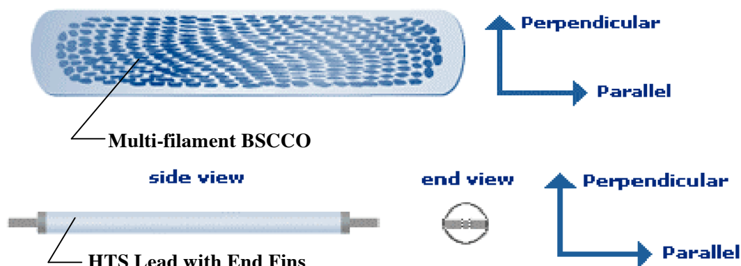
Figure 2. Examples of Favorable Field Orientation (parallel to the flat faces of the conductor) and unfavorable field orientations (perpendicular to the conductor flat face) for leads made for oriented BSSCO tape type HTS superconductor. The lead end fins indicate the conductor flat face direction. (With permission from HTS-110 Inc.)
