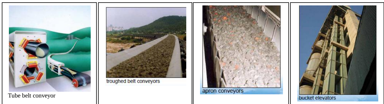
Figure 29. Mechanical transport systems (Hock 2008)
