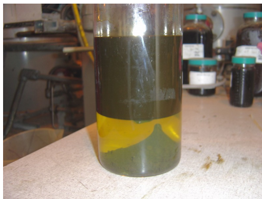
Figure 5: Sleeve contents after removal from reactor during a catalytic run at TDP
