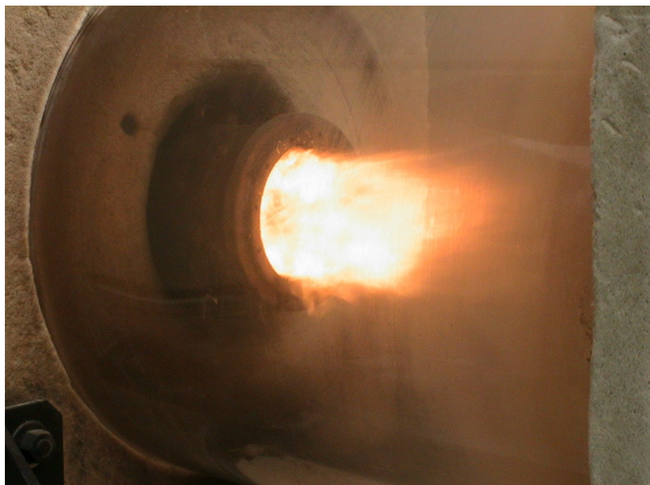
Figure 3: Flame produced by No.2 oil – quartz combustion chamber
