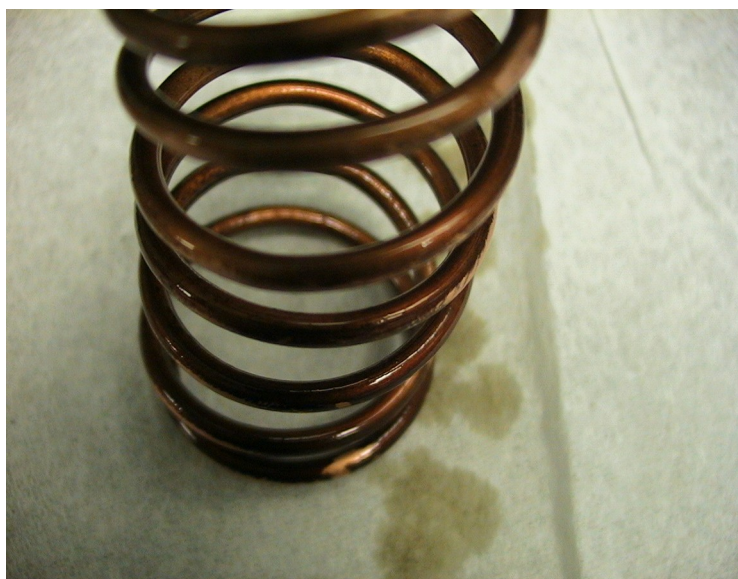
Figure 5 copper coil after 2 months exposure in 50/50 fuel blend
