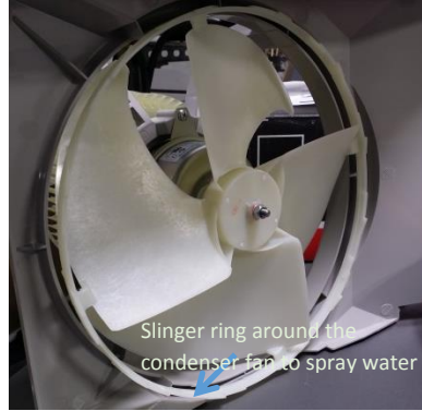
Figure 4: Slinger ring on condenser fan
