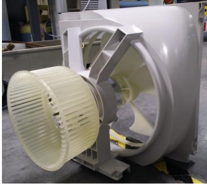
Figure 3: Single axis blower/fan
